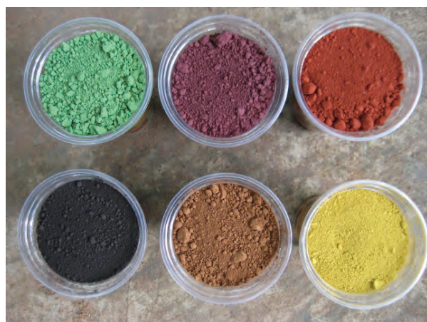
Fig.4.4 Pigment for adjustment the mortar color(JASA)
