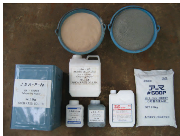
Fig.4.3 Cementitious materials for stone repair(JASA)
